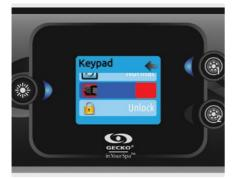
With the in.k500 equipped with a selectable rim light color modul: If the "RGB backlight" option is enabled in the spa configuration an option will appear to allow selection of the keypad rim light color.
